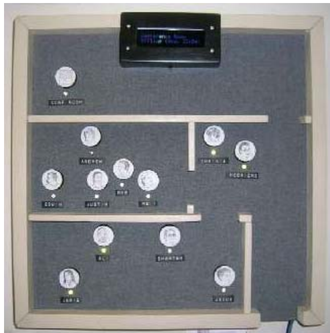
Figure 1: The Online Enlightenment lab presence notification system. Status lights on the display turn on and off (but do not blink!) to reflect the presence of lab members.
