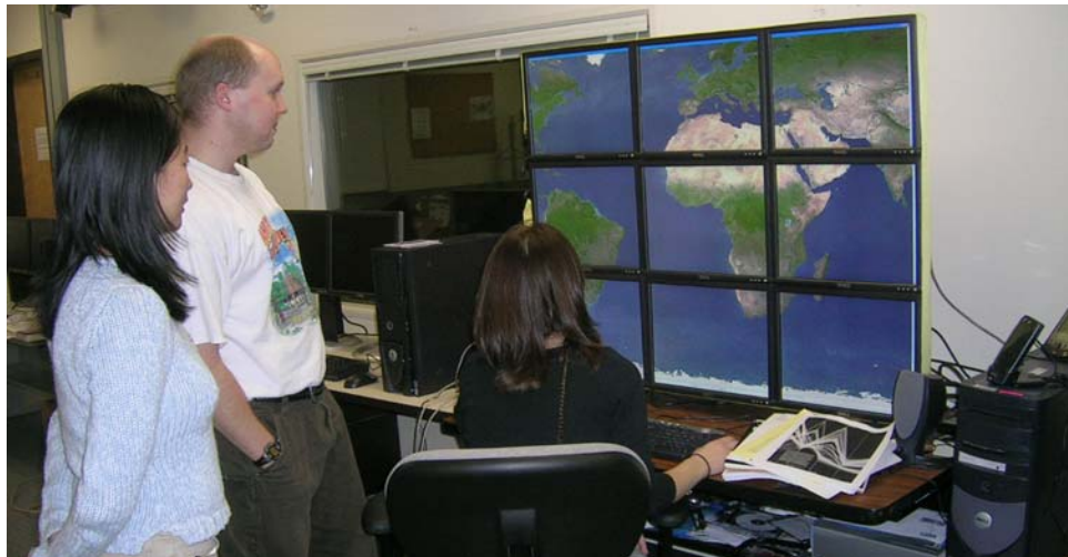
Figure 3: Nine screen display used in the IRVE experiment. Participants either worked in the virtual environment shown on a single monitor or shown on all nine monitors.
