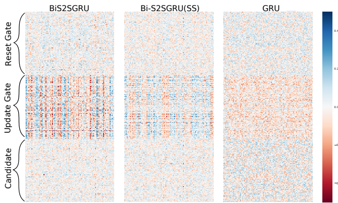
Fig. 8: Heatmap of GRU weight matrices (reset gate, update gate and candidate). We see that Bi-Seq2Seq models learn sparser weights than simple recurrent models. Also the update gate weight matrix in Bi-Seq2Seq models shows definite patterns, with the scheduled sampling variant (Bi-S2S(SS)) being sparser.
