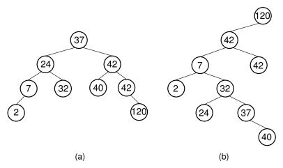
**Figure 5.13** Two Binary Search Trees for a collection of values. Tree (a) results if values are inserted in the order 37, 24, 42, 7, 2, 40, 42, 32, 120. Tree (b) results if the same values are inserted in the order 120, 42, 42, 7, 2, 32, 37, 24, 40.
