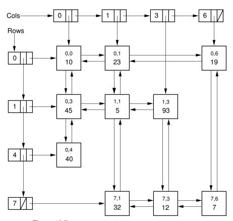
**Figure 12.7** The orthogonal list sparse matrix representation.
