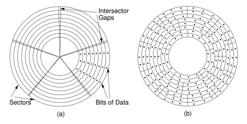
**Figure 8.3** The organization of a disk platter. Dots indicate density of information. (a) Nominal arrangement of tracks showing decreasing data density when moving outward from the center of the disk. (b) A "zoned" arrangement with the sector size and density periodically reset in tracks further away from the center.
