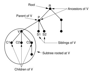
**Figure 6.1** Notation for general trees. Node P is the parent of nodes V, SI, and S2. Thus, V, SI, and S2 are children of P. Nodes R and P are ancestors of V. Nodes V, SI, and S2 are called **siblings**. The oval surrounds the subtree having V as its root.
