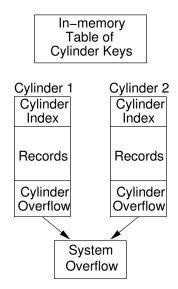
**Figure 10.6** Illustration of the ISAM indexing system.
