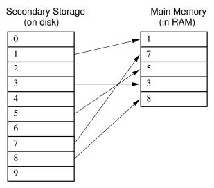
**Figure 8.5** An illustration of virtual memory. The complete collection of information resides in the slower, secondary storage (on disk). Those sectors recently accessed are held in the fast main memory (in RAM). In this example, copies of Sectors 1, 7, 5, 3, and 8 from secondary storage are currently stored in the main memory. If a memory access to Sector 9 is received, one of the sectors currently in main memory must be replaced.
