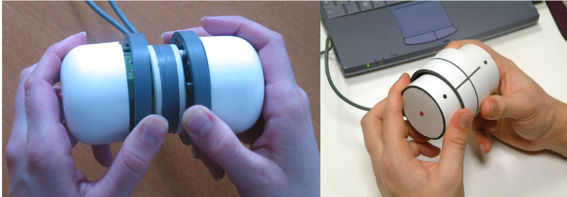
Figure 6: The Round Bone (left) and the Tire (right). Both devices are built from elastic SpaceMouse sensors.
