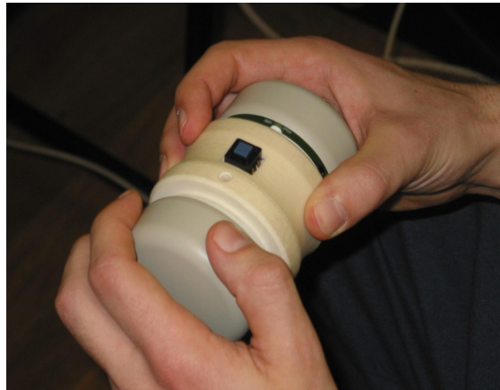
Figure 3: The YoYo consist of two SpaceMouse sensors attached to a grip in the middle
