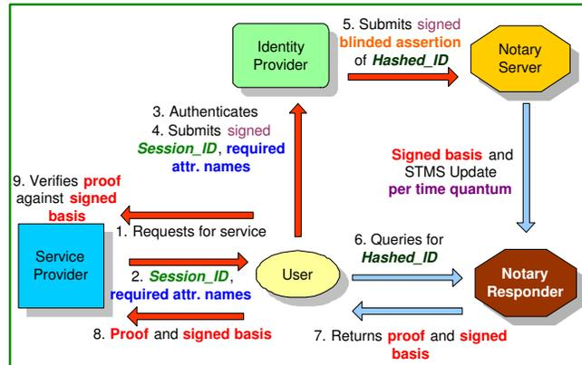
**Fig. 3.** A schematic drawing of the STMS implemented notarized federated identity management protocol. At each time quantum, the notary source sends the signed basis and updates of the authenticated dictionary to the notary responder. The notary responder answers a query for assertion by returning the signed basis and the proof corresponding to the queried element.
