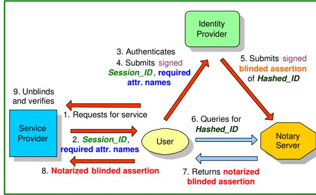
**Fig. 1.** Overview of the notarized federated identity management protocol. Red lines represent secure communication channels. Blue lines indicate that secure channels are *not* required.
