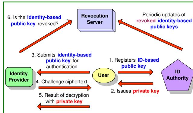
**Fig. 4.** A diagram of the ID-based authentication protocol. Identity information is used as the public key in this protocol. This identity information *cannot* be used by others for impersonation without knowing the corresponding private key.
