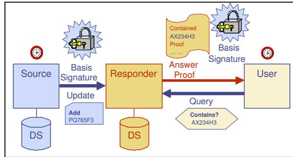
**Fig. 2.** Overview of STMS. The source pushes updates containing a signed basis to the responder. The responder then answers user queries with a proof of the answer, and a copy of the signed basis from the source.
