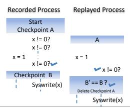
**Figure 2.** A race that produces the same program state irrespective of the order between the racing memory operations. Although the number of reads executed by the replayed process is different from the recorded process causing a transient divergence, the executions eventually converge to the same program state.
