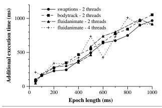
Figure 5. Impact of epoch interval on rollback overhead
