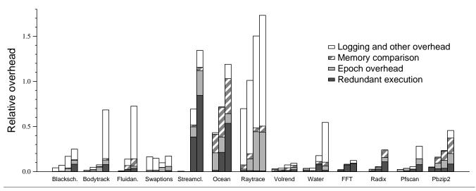
**Figure 4.** Breakdown of overhead per benchmark. For most benchmarks, results are presented for 1, 2, 3, and 4 threads (left to right). For Fluidanimate, Ocean, FFT, and Radix, results are presented for 1, 2, and 4 threads.
