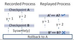
**Figure 3.** An execution with a data race that causes the replayed process to produce a memory state different from that of the recorded process. The divergence check fails and the two processes are rolled back to an earlier checkpoint.
