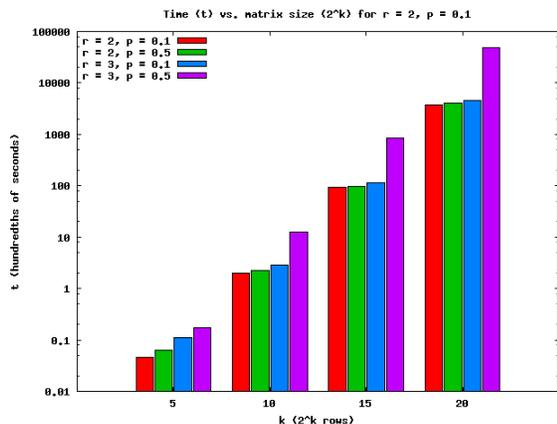
Figure 6: Observed running time  $t$  as we vary  $k$  ( $2^k$  rows) and fix probability  $p$  and column width  $r$ .
