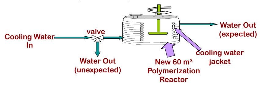
He found that a valve had been carelessly switched to the wrong position, thereby diverting cooling water away from the reactor so that virtually no cooling took place.
