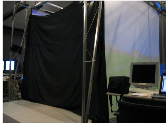
Fig. 2: CAVE in the low-stimulus GBD condition: a black cloth covering the missing wall.
