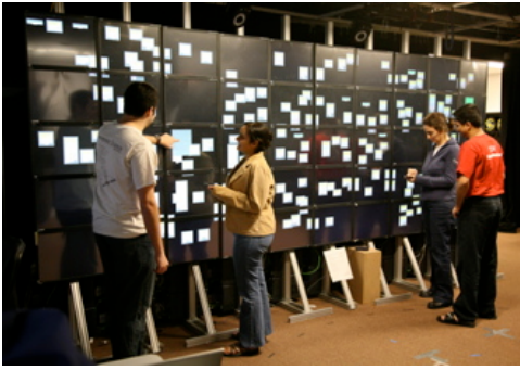
Figure 1: Prototype of collaborative tool for creating affinity diagrams using a wall sized display and PDAs
