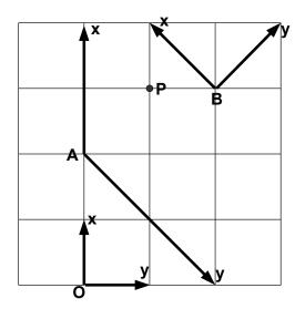
Notation:  $M_{ST}$  is a 3x3 homogeneous matrix that transforms points from coordinate system S to coordinate system T.
