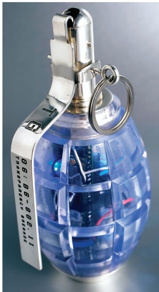
Figure 2. Transparency Grenade. The transparent shell contains a microcomputer, wireless antenna, and microphone that can securely and anonymously stream captured network traffic and audio to a server for subsequent analysis. (Courtesy of Khuong Bismuth.)
