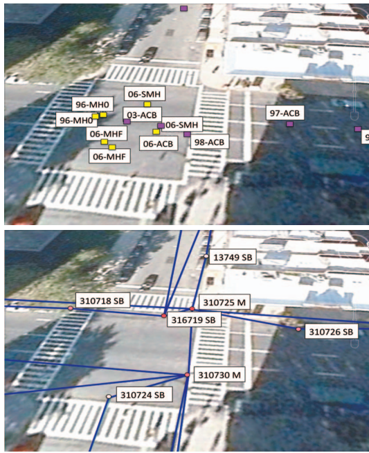
Fig. 22. Images from the manhole events visualization tool, where labels were enlarged for clarity. Top: Geocoded ticket addresses, colored by trouble type. Yellow indicates a serious event type, purple indicates a potential precursor. If the user clicks on a ticket, the full ticket text is displayed. Bottom: Manholes and main cables within the same location, where manholes are colored by predicted vulnerability. Note that a ticket within the top figure does not necessarily correspond to the nearest manhole on the bottom figure.
