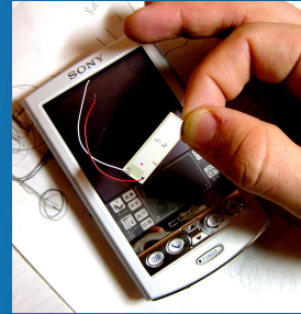
Piezo actuator for touch screens
