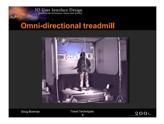
The image shows the omni-directional treadmill, developed by SARCOS corporation, which allows the user to walk in any direction on the horizontal plane. It works very well for slow, controlled walking, but has usability problems during sudden stops and starts, quick changes of direction, etc. due to the fact that it must actively try to keep the user near the center of the device. See Darken, Cockayne, & Carmein, UIST 1997, pp. 213-221 for more details.
