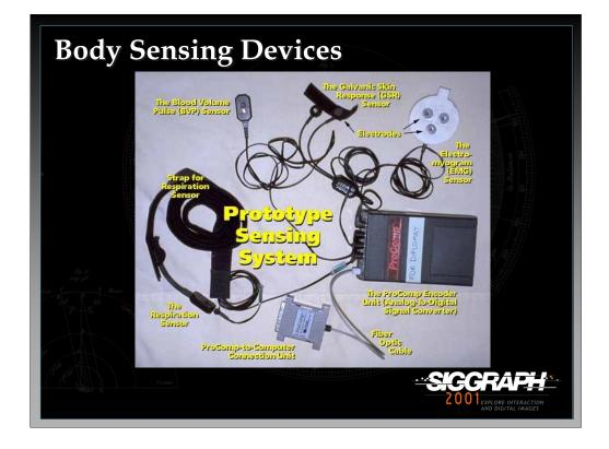
The MIT Media Lab's affective computing group has developed a Prototype Physiological Sensing System which includes a Galvanic Skin Response sensor, a Blood Volume Pulse sensor, a Respiration sensor, and an Electromyogram. By using this prototype, interface developers can monitor a user's emotional state to dynamically modify an application's interface to better fit the user's needs.
