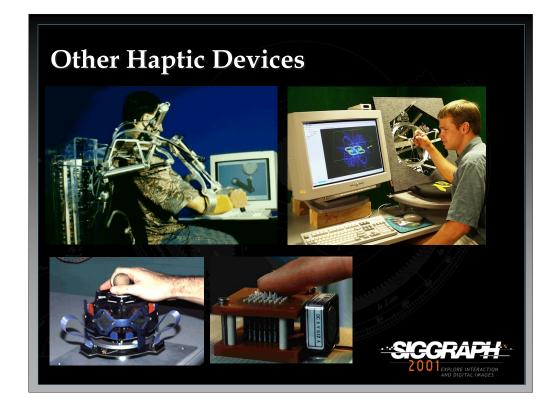
There are many different haptic devices that are being developed in research labs around the world. The slide shows from top to bottom, left to right the Pneumatic Master Arm from Southern Methodist University, a 5 DOF haptic device from the University of Colorado, a magnetic levitation haptic interface from Carnegie Mellon University, and a tactile display from the Karlsruhe Research Center in Germany.
