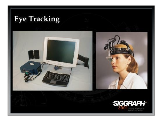
Eye tracking systems provide applications with knowledge of the user's gaze direction. This information opens the door to a number of interesting interaction techniques such as eye directed selection and manipulation. The figure on the left shows the Eyegaze system, a non-intrusive approach which uses an infra-red source that reflects off of the pupil, developed by LC Technologies. The figure on the right shows iView, a head-mounted eye tracking device developed by SensoMotoric Instruments.
