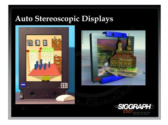
Other visual output devices use lenticular, volumetric, and holographic display technology. Most of these technologies are expensive and in the early stages of development so they are rarely utilized in mainstream 3D interfaces. However, once these technologies become more affordable and the technology has progressed sufficiently, a number of interesting interface issues will arise.
