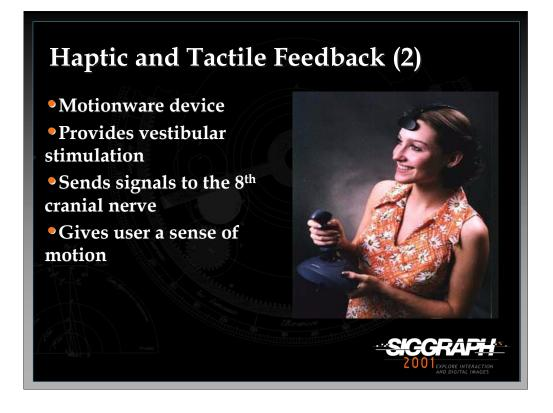
Another type of tactile feedback device is Motionware being developed by Virtual Motion. Motionware sends electrical current to the 8th cranial nerve located behind the wearer's ear. Sending these electrical signals to the 8th cranial nerve provides the user with vestibular stimulation which can mimic the sense of motion. The device will be priced at around \$100.
