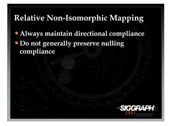
In contrast to absolute mappings, relative non-isomorphic mappings always maintain directional compliance and do not generally preserve nulling compliance. This means that relative non-isomorphic mappings can be very efficient in manual control tasks assuming the multiple DOF input device has the right form factor. The right form factor in this case is the device can be freely rotated in the fingers.
