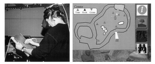
Figure 6. Physical (left) and virtual (right) views of the pen & tablet interaction metaphor
