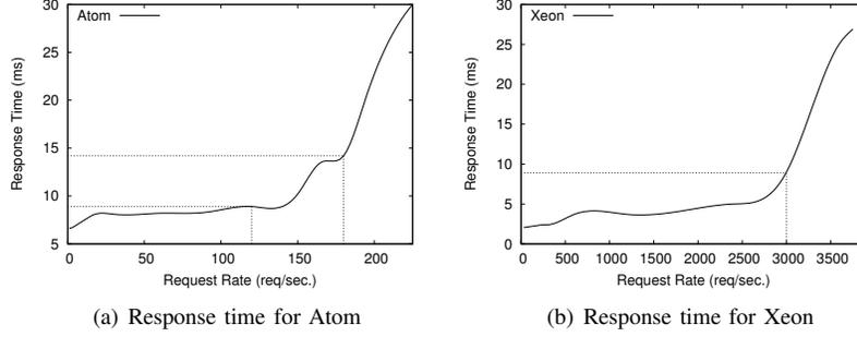
**Fig. 4:** Response time profiles for Atom and Xeon for Dynamic Content Server.
