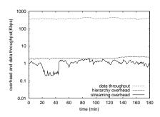
**Fig. 8.** Representative scenario: overhead at clients in MetaStream
