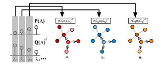
Fig. 10. Illustration of B-3: A rational function maps the eigenvalues to new values.
