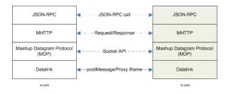
Figure 3. Communication stack in OMOS. The arrows and their texts are the communication methods for the layers. Note that all the communications between two mashlets take place within the end user's browser.
