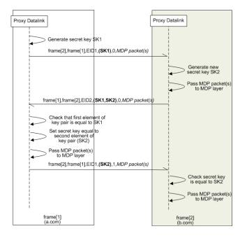
Figure 4. Key establishment protocol between two mashlets, frame[1] from a.com and frame[2] from b.com, through Datalink layer.
