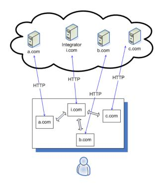
Figure 1. Client-side mashup architecture. The rectangle represents the browser on the client's local computer where contents from heterogeneous data sources such as a.com and b.com are mashed up.
