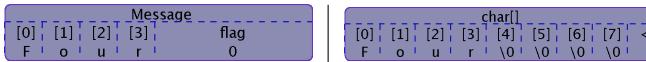
Figure 11: The buffer overflow overwrote the least significant byte of 'flag,' changing its value to zero. A user can observe the overlap between flag and the zero sentinel placed by strcpy() when copying the string "Four" into a buffer that was too small.
