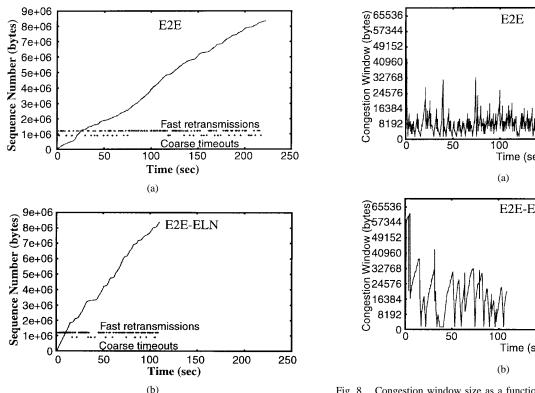
Fig. 7. Packet sequence traces for E2E (TCP Reno) and E2E-ELN. The top row of horizontal dots shows the times when fast retransmissions occur; the bottom row shows the coarse timeouts.
