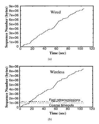
Fig. 10. Packet sequence trace for the wind and wireless parts of the SPLIT protocol. The wireless part has two rows of horizontal dots: the top one shows the times of fast retransmissions, and the bottom one the times of the timeout-based ones.
