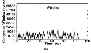
Fig. 11. Congestion window sizes as a function of time for the wired and wireless parts of the split TCP connection. The wired sender never sees any losses, and maintains a 64-kbyte congestion window. However, the wireless TCP connection's congestion window fluctuates rapidly.
