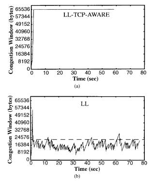
Fig. 4. Congestion window size for link-layer protocols in wide-area tests. The horizontal dashed line in the LL graph shows the 23000 byte WAN bandwidth-delay product.
