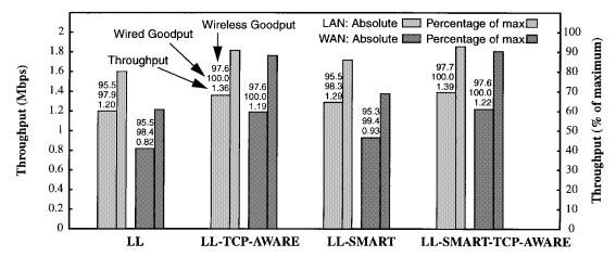
Fig. 3. Performance of link-layer protocols: bit-error rate =  $1.9 \times 10^{-6}$  (1 error/65536 bytes), socket buffer size = 32 kbytes. For each case, there are two bars: the thick one corresponds to the scale on the left and denotes the throughput in megabits per second; the thin one corresponds to the scale on the right and shows the throughput as a percentage of the maximum, i.e., in the absence of wireless errors (1.5 Mb/s in the LAN environment and 1.35 Mb/s in the WAN environment).
