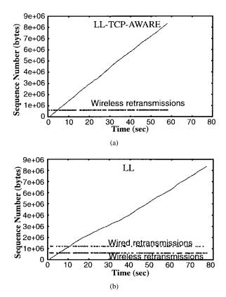
Fig. 5. Packet sequence traces for LL-TCP-AWARE and LL. No coarse timeouts occur in either case. For LL-TCP-AWARE, the horizontal row of dots shows the times of wireless link retransmissions. For LL, the top row shows sender fast retransmission times, and the bottom row shows both local wireless and sender retransmissions.
