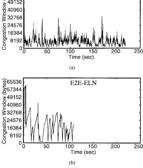
Fig. 8. Congestion window size as a function of time for E2E (TCP Reno) and E2E-ELN. This figure clearly shows the utility of ELN in preventing rapid fluctuations, thereby maintaining a larger average congestion windows size.
