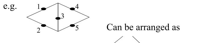
A parallel connection of series structures
