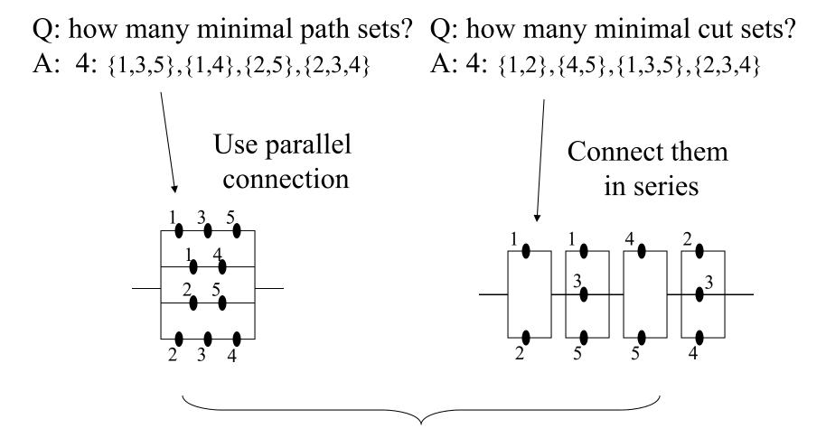
There are series-parallel diagrams with common components
