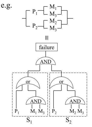
2 processors: P<sub>1</sub> & P<sub>2</sub> 3 memory modules: M<sub>1</sub>, M<sub>2</sub> & M<sub>3</sub>
