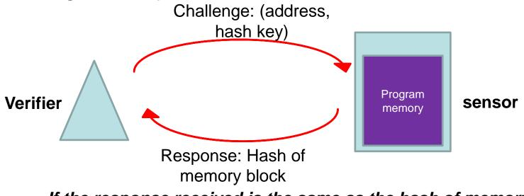
If the response received is the same as the hash of memory block computed by the verifier, then the sensor is clean
