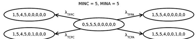
Fig. 6. Attrition failure in the underlying semi-Markov model.
