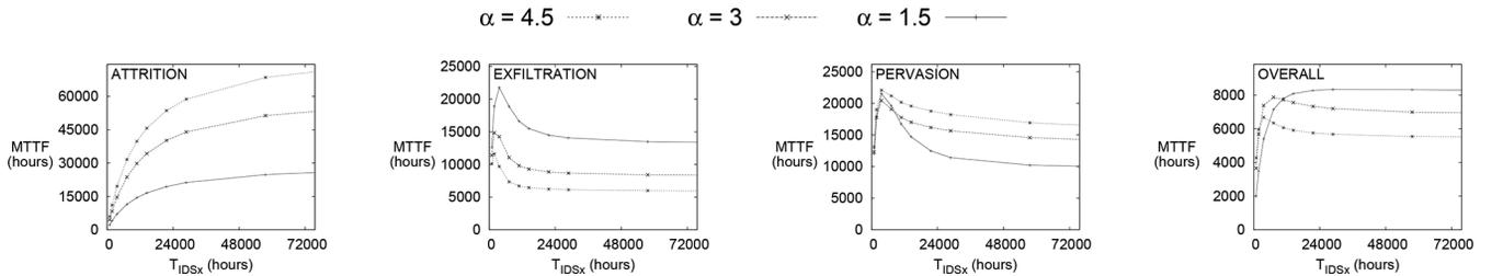
Fig. 12. MTTF vs.  $T_{IDSx}$  with varying  $\alpha$  ( $\mathcal{P}_{fn} = 0.1$ ,  $\mathcal{P}_{fp} = 0.2$ ,  $\lambda_x = 1/(2400\text{ days})$ ).
