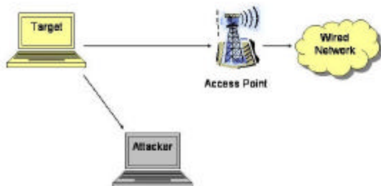
Figure 1 Illustration of passive eavesdropping. The attacker simply listens in on the radio broadcasts of the target and wireless LAN.
