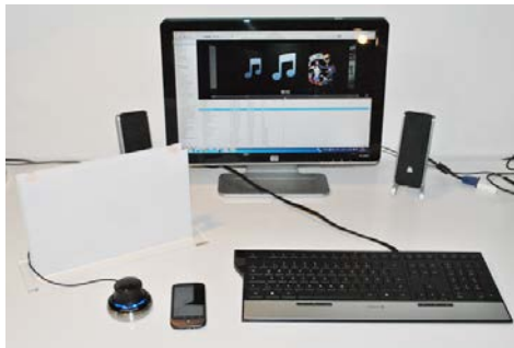
Figure 3. The Peripheral Audio Player supports alternatively free hand gestures (white box hides the tracking), tangible interaction (3D mouse) and touch gestures (through a mobile phone).
