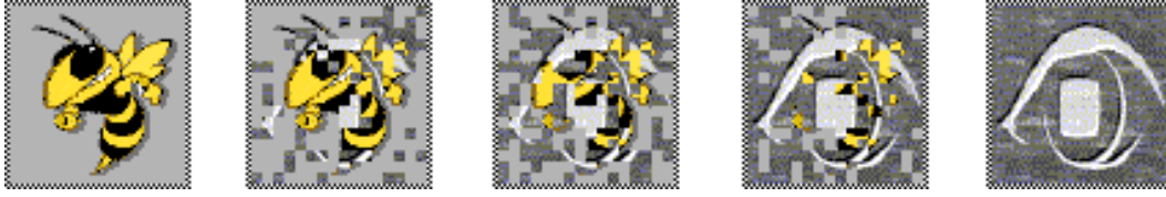
Figure 8: A time-lapse series of the fade widget for two images. Rather than perform compute-intensive calculations to achieve a fading effect, the original image is broken into pieces, and the pieces of the original are gradually replaced with pieces of the final.
