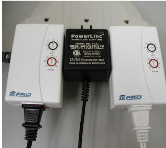
Figure 2: X10 components used in constructing a RWI. The black box is the Powerline adaptor that allows a computer to send signals via the serial port through power lines. The white boxes are X10 receivers into which appliances can be plugged. Each receiver has one of 256 available codes.
