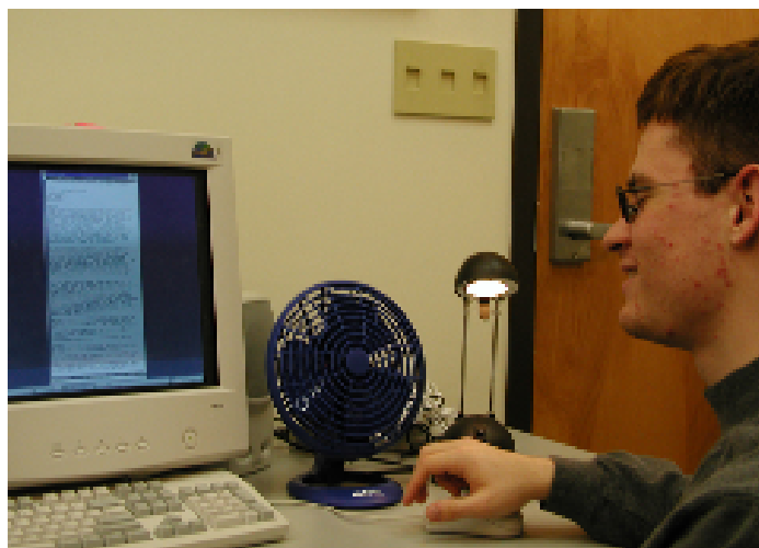
Figure 4: The weather monitor RWI. The brightness of the lamp reflects the current temperature relative to the expected temperature for the region, and the fan reflects precipitation. The RWIs are situated by the door as a reminder when leaving to consider bringing a jacket or umbrella.
