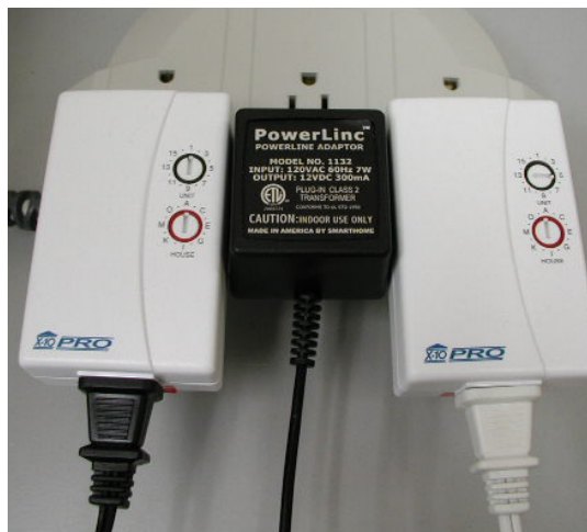
Fig. 1. X10 components used in constructing a RWI. The black box is the Powerline interface that allows a computer to send signals via the serial port through the power lines. The white boxes are X10 receivers into which appliances can be plugged. Each receiver should have a different code, with up to 256 different codes available.
