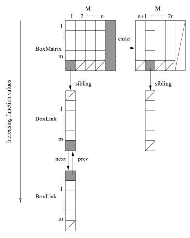
Figure 2. Box structures comprised of HyperBoxes.
