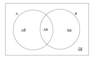
$$\begin{array}{ll} support(A\overline{B}) &= support(A) - support(AB) \\ support(\overline{AB}) &= support(B) - support(AB) \\ support(\overline{AB}) &= N - support(A) - support(B) + support(AB) \\ support(AB) &= support(AB) \\ N = support(\emptyset) \end{array}$$
