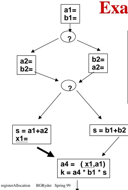
Variable renaming may let us eliminate some interferences. This graph has no interference between x1 and a1. SSA-form: each variable use is reached by only one definition.
