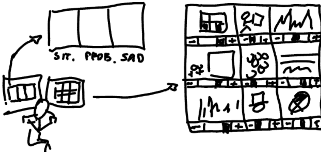
Figure 1: A sketch of the PIC-UP tool, used by a designer pictured in the lower left on a dual-monitor computer. On the left monitor is displayed a storyboard, perhaps chosen by a project design lead based on requirements from a client. On the right monitor is displayed a grid of pictures identified from the claims library by PIC-UP—based on a relevance calculation for the domain, the stage of action of the currently selected storyboard pane, and designer input on relevance of and interest in the currently displayed images. The designer’s task is to create a new design storyboard, addressing issues in the problem storyboard with inspiration from pictures.
