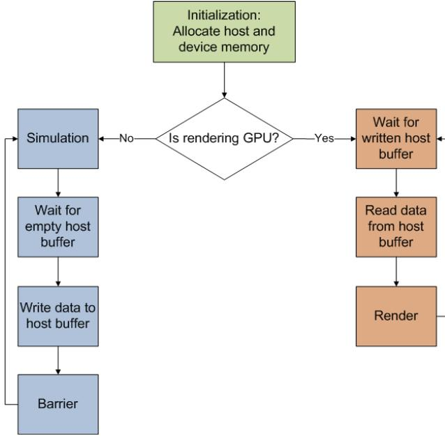
**Fig. 5** The distributed scheduling algorithm for each GPU in our data-driven load balancing approach.
