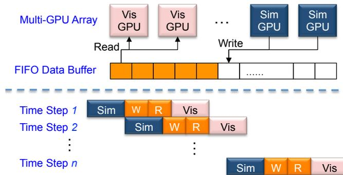
**Fig. 1** Top figure shows the multi-GPU configuration used in an in-situ visualization application, where simulation GPUs and visualization GPUs synchronize the work in a pipeline fashion with the support of a FIFO data buffer. Bottom figure illustrates the pipelining stages in the application.
