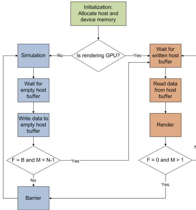
**Fig. 13** This flowchart shows the execution and task switching for dynamic load balancing.  $F$  is the number of host buffers,  $B$  is the maximum number of host buffers,  $M$  is the current number of rendering GPUs, and  $N$  is the total number of GPUs available for load balancing.
