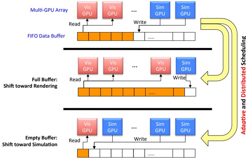
**Fig. 3** The multi-GPU configuration and the problem definition of our load balancing approaches.
