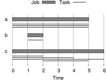
Figure 2. Kinds of jobs in the trace. (a) A *synced* job, (b) a one-task job, and (c) a *non-synced* job.
