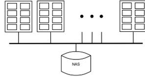
Figure 12. Architecture of a Hadoop cluster with a NAS device.
