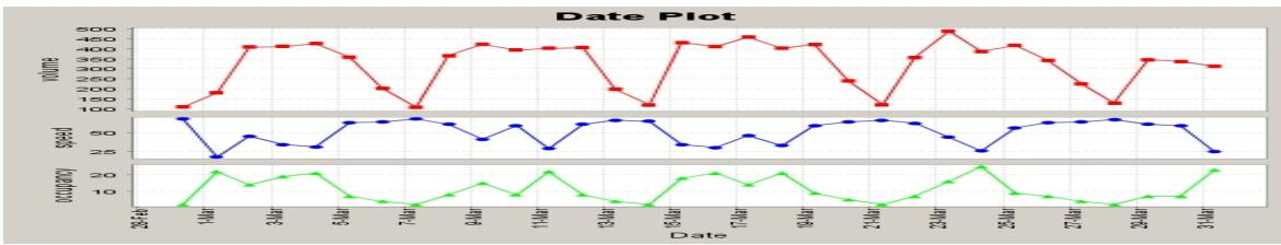
**Figure 2.** Shows speed, volume, and occupancy of a particular station for a specified date range
