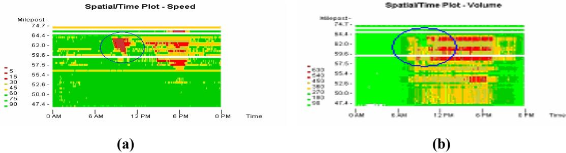
**Figure 4.** Shows speed, volume, and occupancy of a set of station nodes for a specified time of day. Figure above only depicts ‘speed’ and ‘volume’.
