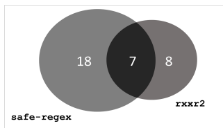
Figure 3: The safe-regex and rxxr2 oracles disagreed on whether many of the regular expressions were vulnerable. Each oracle found true vulnerabilities the other did not.
