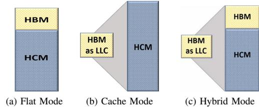
Fig. 1: Memory modes of a heterogeneous system. a) HBM and HCM are two separately addressable memories b) HBM is managed by hardware. Automatic caching is performed. c) HBM is partially available as a separately addressable memory and partly as a hardware managed last level cache (LLC).
