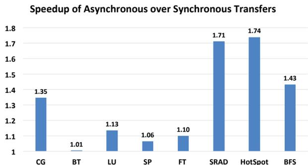
Fig. 5: Speedup achieved by asynchronous transfers over synchronous transfers using dynamic placement strategy.
