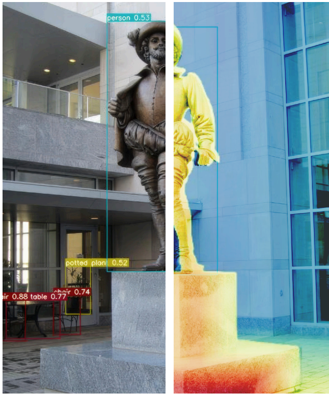
Figure 3. Computer visualization tools. Image processed using YoloV7 for object recognition (left) and DepthAnything-V2 for relative depth estimation (right). Image adapted using CV techniques with permission from Fred Brack, professional audio describer.
