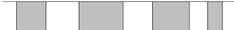
Figure 12.9 Dynamic storage allocation model. Memory is made up of a series of variable-size blocks, some allocated and some free. In this example, shaded areas represent memory currently allocated and unshaded areas represent unused memory available for future allocation.
