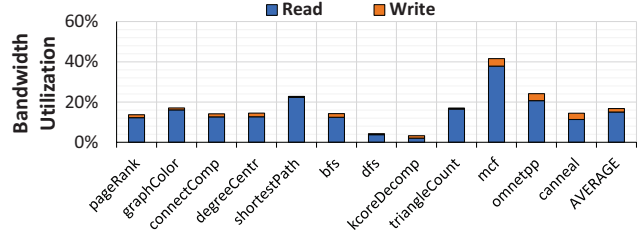
Figure 17: Bandwidth utilization of the evaluated benchmarks during the simulated time window, assuming a conventional system without compression.
