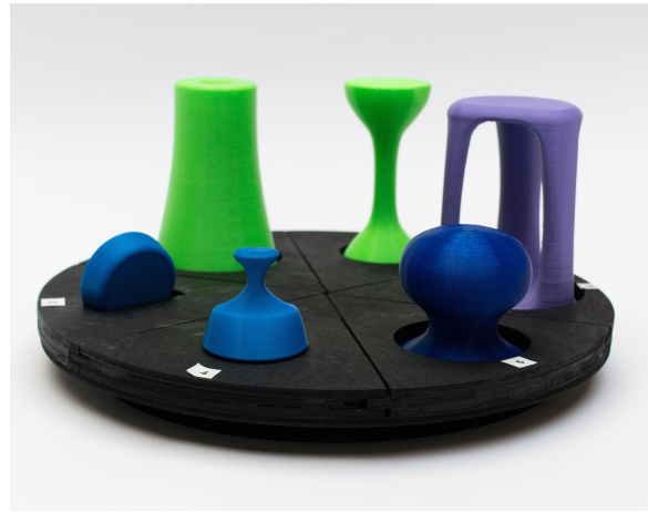
Figure 2. The six objects are stored in a numbered rotatable container to facilitate object identification, object access, and object replacement (each storage slot is unique to each object)
