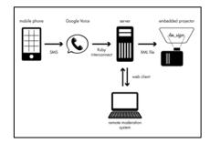
**Figure 3**: System diagram. The web client is used only for administration (eg., removal of profane messages that passed through the blacklist) and is not user-facing.
