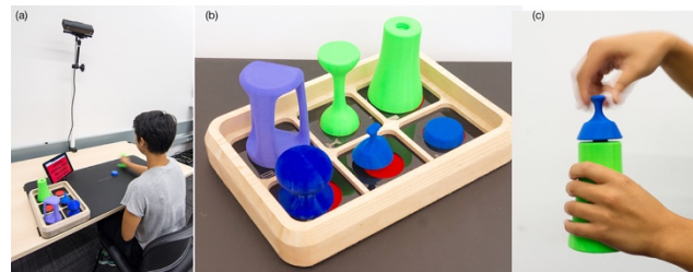
Figure 1. a) The interactive stroke rehabilitation system including mat, objects, tablet and mounted Kinect; b) set of 6 objects; c) combining two objects by screwing together
