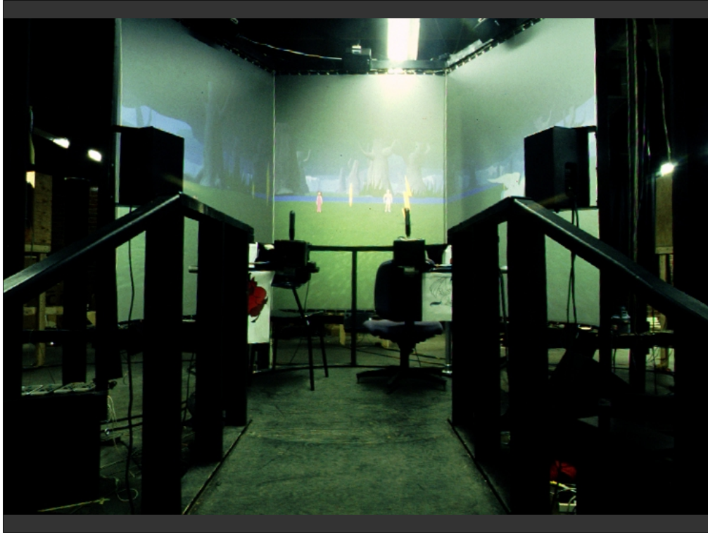
Interior shot of the prototype Hercules CAVE, 5 rear-projection screens (5 sides of a hexagon – only 3 visible in this shot). Projectors were turned on their side for greater vertical aspect ratio. Joysticks are custom designed with 1 inch thick steel shafts down the middle to withstand the rigors of daily use.
