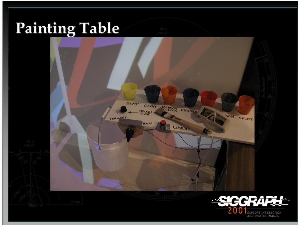
The Painting Table is another example of a discrete input device that is used in the CavePainting application, a system for painting 3D scenes in a virtual environment. The device uses a set of conductive cloth contacts as well as traditional buttons and digital sliders. Users can dip the paint brush prop into the colored cups to change brush strokes. The bucket is used to throw paint around the virtual canvas.
