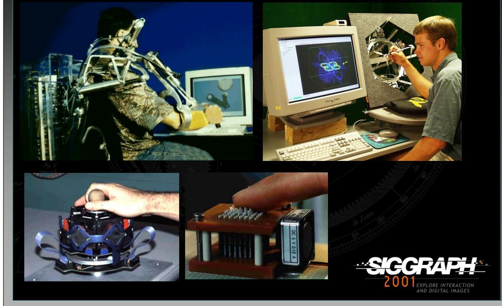
There are many different haptic devices that are being developed in research labs around the world. The slide shows from top to bottom, left to right the Pneumatic Master Arm from Southern Methodist University, a 5 DOF haptic device from the University of Colorado, a magnetic levitation haptic interface from Carnegie Mellon University, and a tactile display from the Karlsruhe Research Center in Germany.
