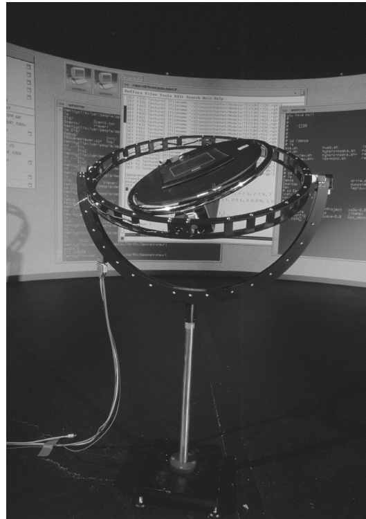
Figure 4.25 The CAT is designed for surround-screen display environments. It combines 6-DOF input with 2D tablet interaction. (Photograph courtesy of the Iparla Team [LaBRI-INRIA])
