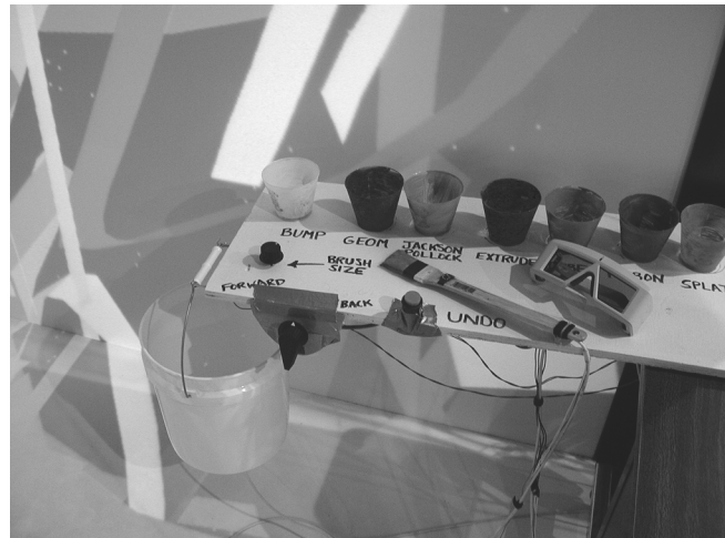
Figure 4.23 The CavePainting Table used in the CavePainting application. (Photograph reprinted from Keefe et al. 2000, © 2001 ACM; reprinted with permission)
