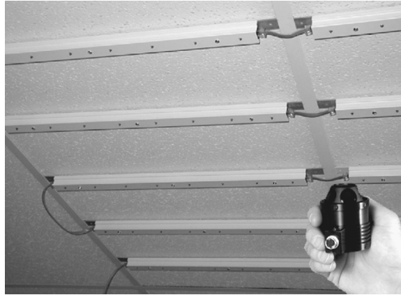
Figure 4.9 The HiBall Tracking System. The LED beacons are mounted on the ceiling, and the camera device is located in the handheld object. (Photograph of the HiBall-3000 Tracker courtesy of 3rd Tech, Inc.)
