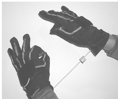
Figure 4.14 A Pinch Glove is a user-worn discrete input device. (Photograph courtesy of Joseph J. LaViola Jr.)
