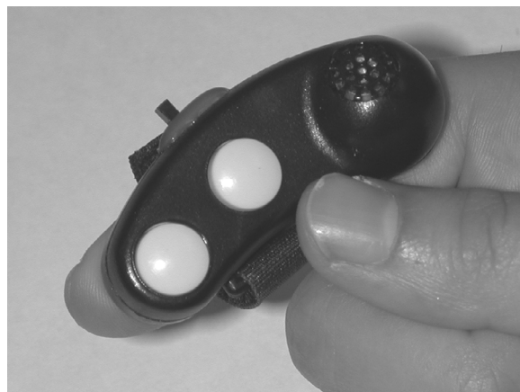
Figure 4.19 The Ring Mouse input device uses acoustic tracking and is worn on a user's index finger. (Photograph courtesy of Joseph J. LaViola Jr.)
