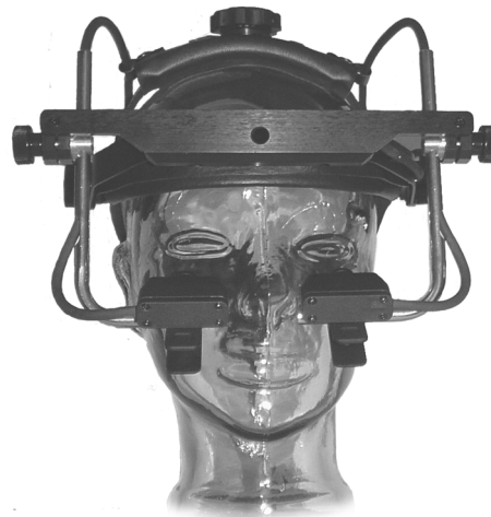
Figure 4.12 This user-worn eye-tracking device uses corneal reflections and pupil tracking to determine eye position. (Photograph courtesy of SR Research, Ltd.)
