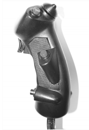
Figure 4.17 A joystick modeled after a flight stick used in 3D VR applications. (Built by VP Integrated Solutions as a large-scale visualization device)
