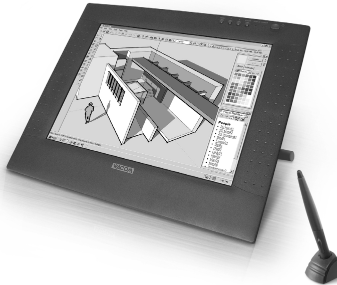
Figure 4.1 A large pen-based LCD tablet allowing the user to draw directly on the screen. (Photograph courtesy of Wacom Technology and @Last Software)
