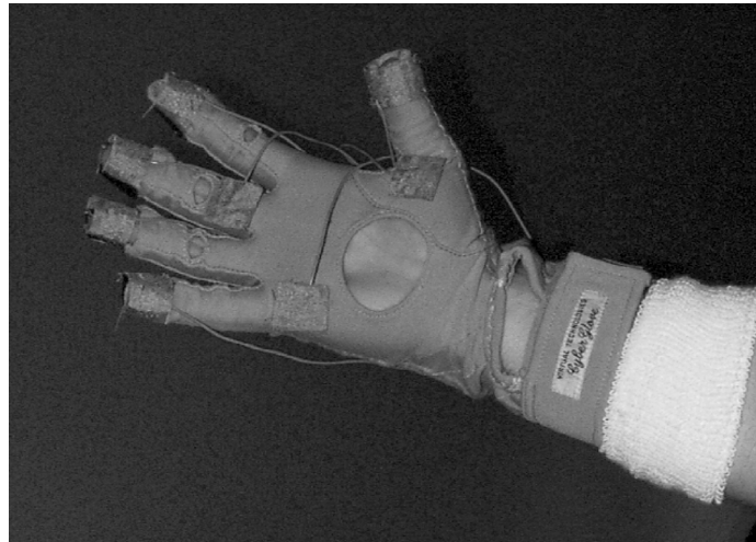
Figure 4.15 The Flex and Pinch input system combines bend-sensing input with discrete buttons. (Photograph courtesy of Joseph J. LaViola Jr.)
