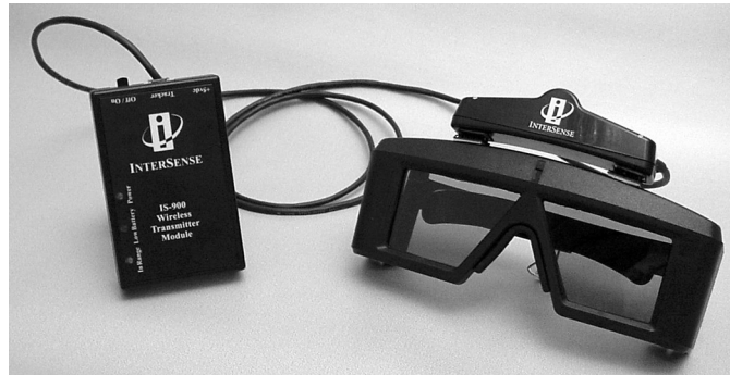
Figure 4.10 A wireless inertial/ultrasonic tracker. (Photograph courtesy of InterSense, Inc.)
