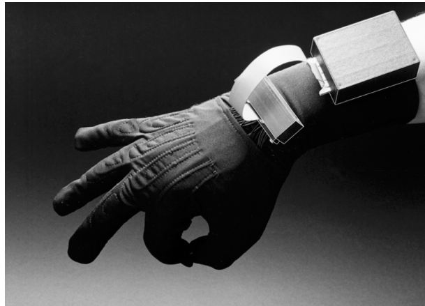
Figure 4.13 A bend-sensing data glove. (Photograph courtesy of Fifth Dimension Technologies, www.5dt.com )
